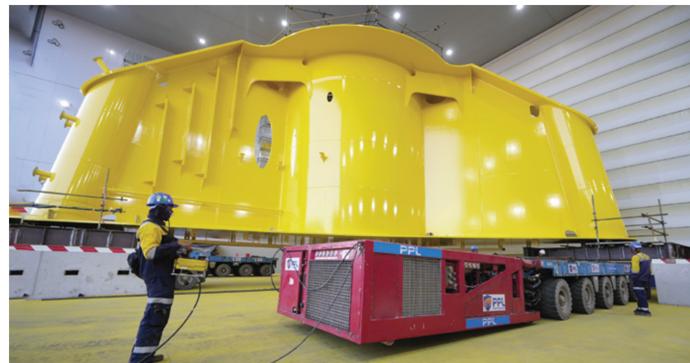
Transition Piece (TP) 21.19 x 19.145 x 10.135 m 379.69 tons
