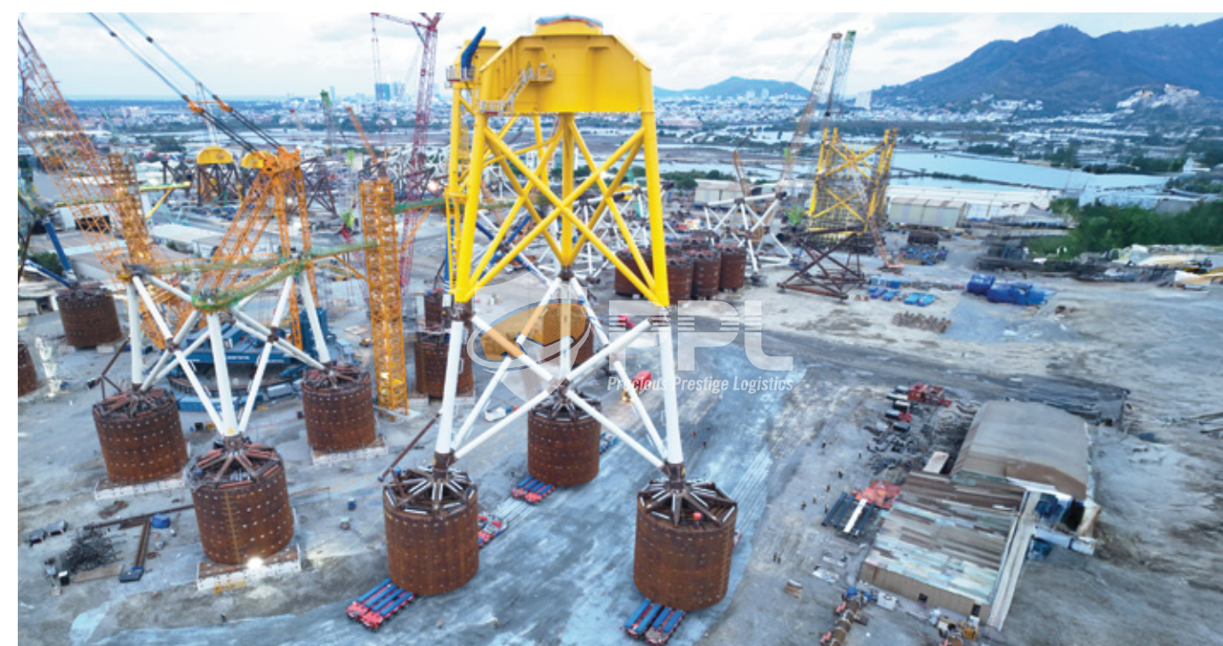
Suction Bucket Jacket 51.596 x 46.566 x 82.040 m 2,387 tons
