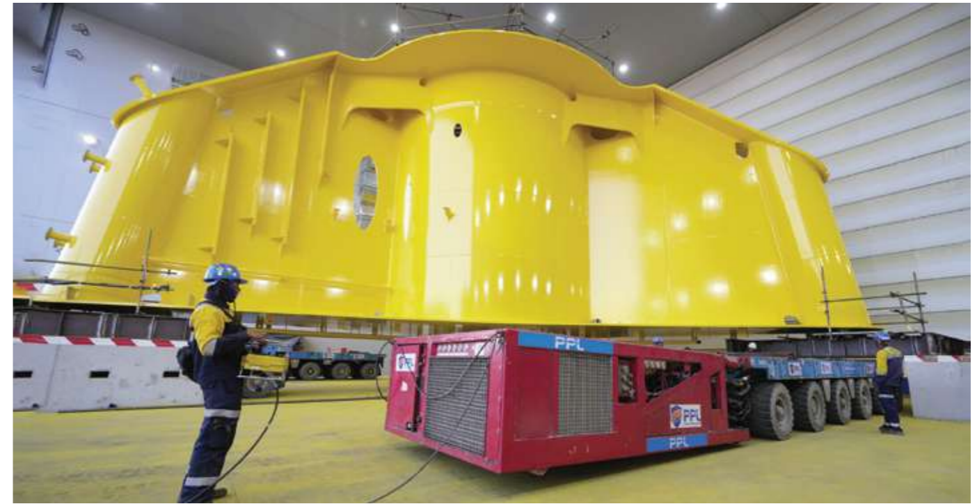
Transition Piece (TP) 21.19 x 19.145 x 10.135 m 379.69 tons
